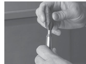
Lightly chamfer the case mouth with a Deburring Tool to remove rough edges for easier bullet seating.
