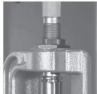
Notice the Sizer Die is adjusted so it contacts the Shell Holder.
